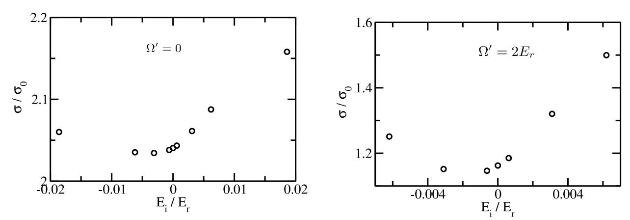
Density spread as a function of initial interaction energy  $E_i$  after evolving time  $1000\hbar/E_r$ .
