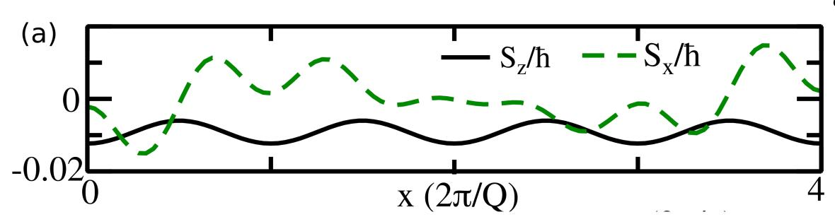
Spin polarization along the x and z direction as a function of x.
